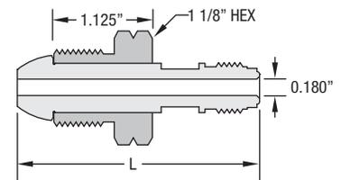
**INLETS X ORBITAL TUBE WELD STUB (INCLUDES SILVER PLATED 303 SS NUT & 316L SS NIPPLE)**
