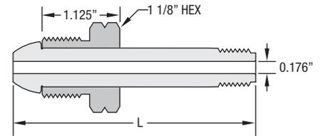
**INLETS X 1/4 MALE FACE SEAL (INCLUDES 303 SS NUT & 316L SS NIPPLE)**
