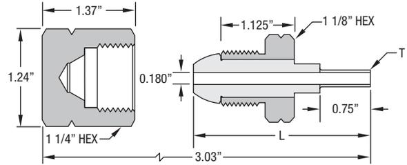
**COMPLETE PIGTAIL CONNECTION X 1/4 MALE FACE SEAL (INCLUDES 303 SS NUT, 316L SS NIPPLE & 303 SS BLANK CAP)**
