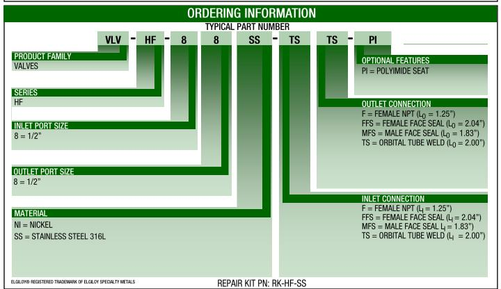
3 PORT, 4 PORT AND CUSTOM CONFIGURATIONS ARE AVAILABLE ON REQUEST. ALSO AVAILABLE WITH PNUEMATIC OPERATOR, SEE HP1KHF SERIES.
