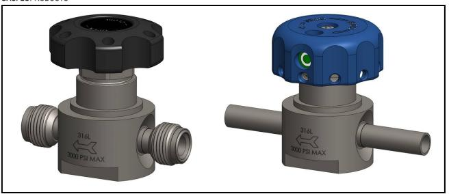
GasFlo Products HF Series valves are a high pressure, high flow design. This spring type, diaphragm, bar stock valve body can be easily field maintained with an economical re-build kit. The HF Series provides an extended service life, positive shut off and smooth operation in 1/2" applications with pressure ranges from vacuum to 3000 psig.
